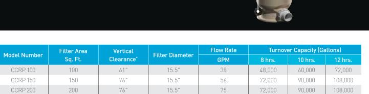
\* Required clearance to remove filter elements
